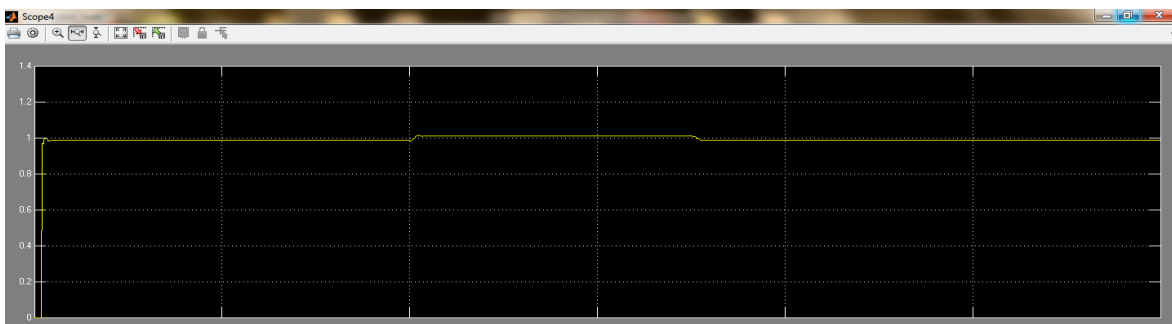
Fig. 9(b). Load Voltage during Outage with USSC
